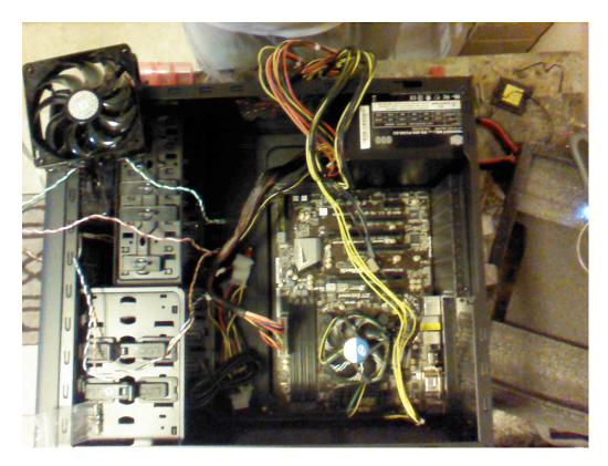
9. Break out the thermal paste and heat sink, apply a pea-size dot of the thermal paste on top of the CPU, slowly and evenly spread the paste on the CPU by pressing down on the paste with the heat sink making sure that none of it spills onto the motherboard, this can break/short your motherboard
